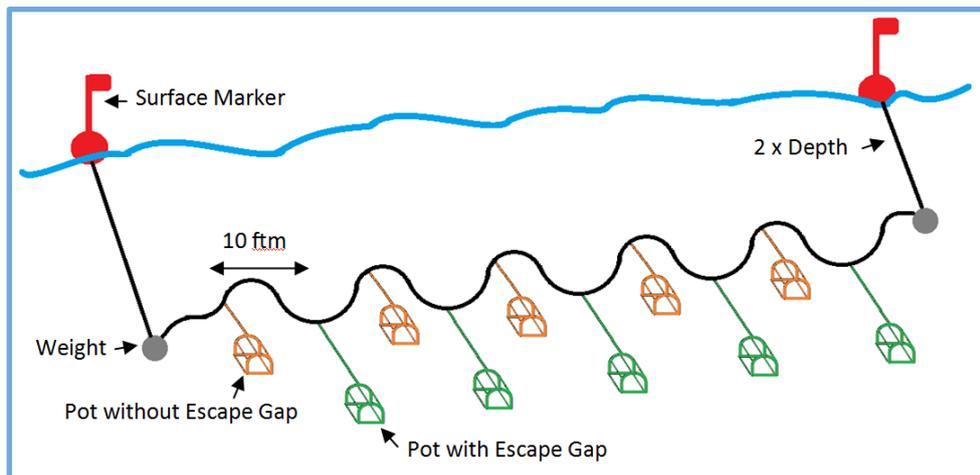
**Figure 1.** Diagram outlining the fleet set-up used during the NIFCA Escape Gap survey.
